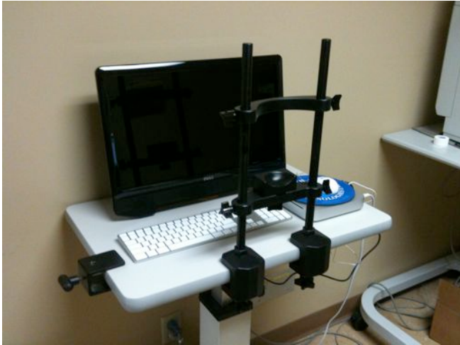
Figure 1. Examination station setup at one of six established test sites to date for the Internet-based, comprehensive visual field test & diagnosis system. Each test site is equipped with a standardized set of hardware comprising an Apple Mac mini computer, a head-chin rest, and a touch-sensitive computer monitor.
